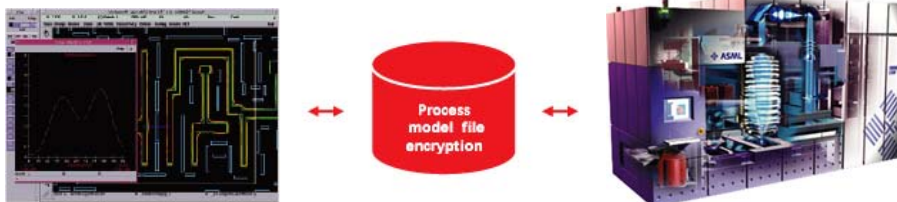
図2: Process model file (PMF) as central, seamless and secure background communication modality to pre- and post-tapeout RET verification with real-world process model information.
